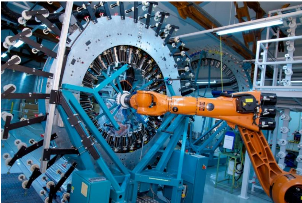
Automatic Wrapping of Tie Rods.
